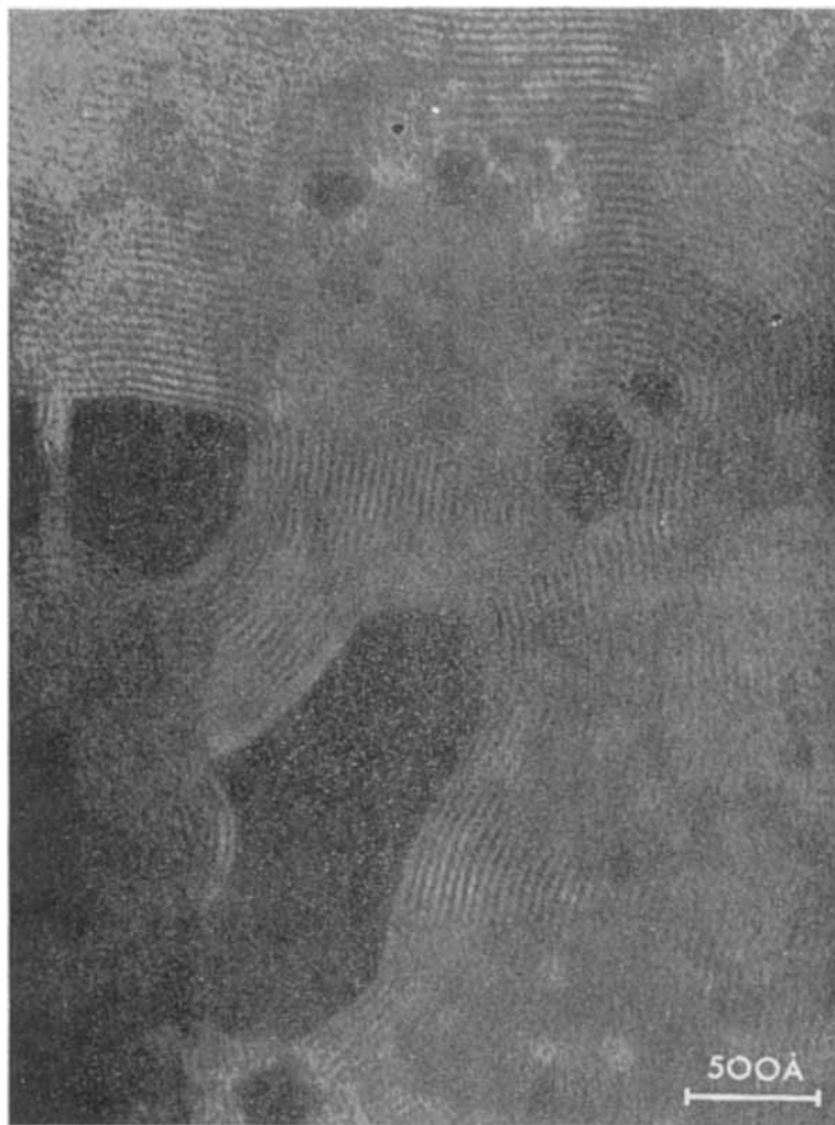
Figure 7. Negatively stained crystals + neat phase from didecanoyl lecithin + water system.
